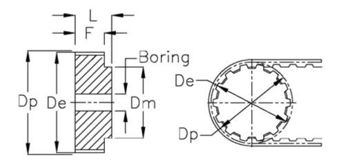
Type = AT10Belt width = - 50 mm Weight = 2.83= 150.95De Dm = 95 = 76.4Dp F = 56 L = 66 Pre-drilled = 16 Tooth number = 48
